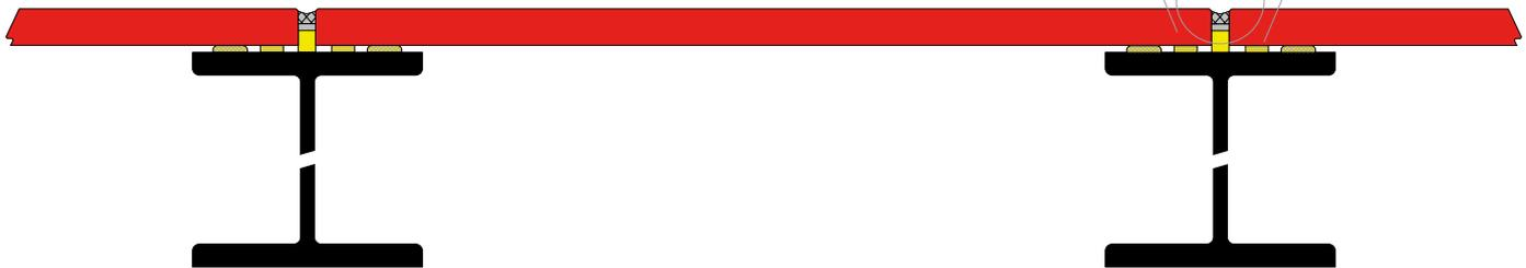
BALKONBODENPLATTE AUF STAHLTRÄGER VERDECKT BEFESTIGT (GEKLEBT)
